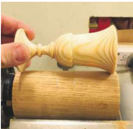
▲ Pic.7 Hold the pattern up against the base section. Even though Les is not making a pair he is pleased with the shape of the pine one so doesn't intend to change it too much
